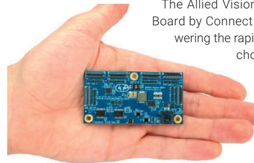
The Allied Vision MIPI Camera Board by Connect Tech is empowering the rapid integration of chosen sensors within an AGX Xavier project. The Camera Board has a small footprint (75x40,2mm)
