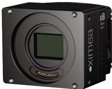
parameters close to sCMOS performance. The 8K consists of 9344x7000 which is the world's highest resolution sensor with Global shutter. For overall heat dissipation reduction and better noise results, the cameras are equipped with a fan cooler which can be removed and replaced with a heatsink or water cooling system. The camera has a PCI Express Gen3 interface with the bandwidth of 64Gbits and real data throughput of 7000MB/s. All in a housing of 60x70x40mm and 250g.
